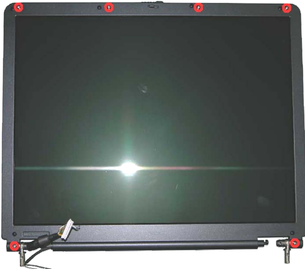
Fig. 17 Removing the rubber covers & screws on the LCD Module
